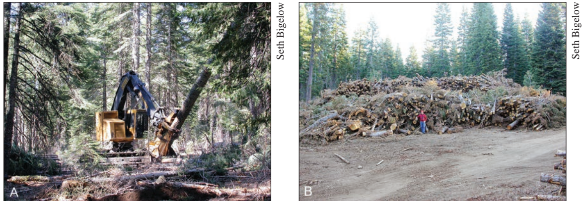
Figure 32—Feller bunchers are commonly used to harvest whole trees during fuel treatments. (A) A swing boom feller buncher can reach out to harvest fuels, eliminating the need to drive to each tree. (B) Whole tree harvest material is often processed at a landing.
