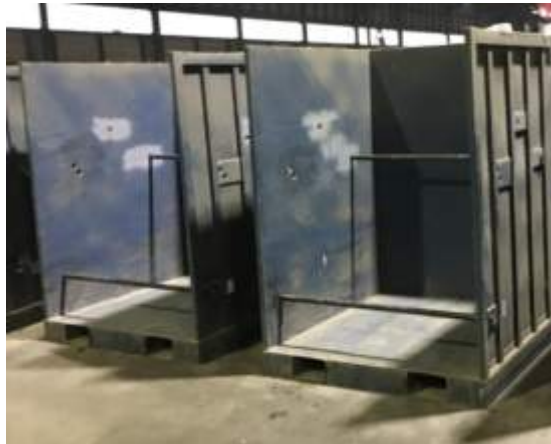
Figure 5.2.3 Example of 3-sided WFS bins
